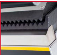
Grease and debris collection gutter
